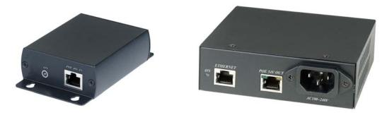
This IP05 POE kit is a cost-effective solution to send data and power over original Ethernet network but eliminates the need of power cable and converter. It is perfect for network application such as IP camera, VoIP and wireless access point This POE kits include two devices, the injector IP05I sends both power and data over signal CAT5 cable to your IP device. The splitter separates the data and power and delivers them to the IP device.
